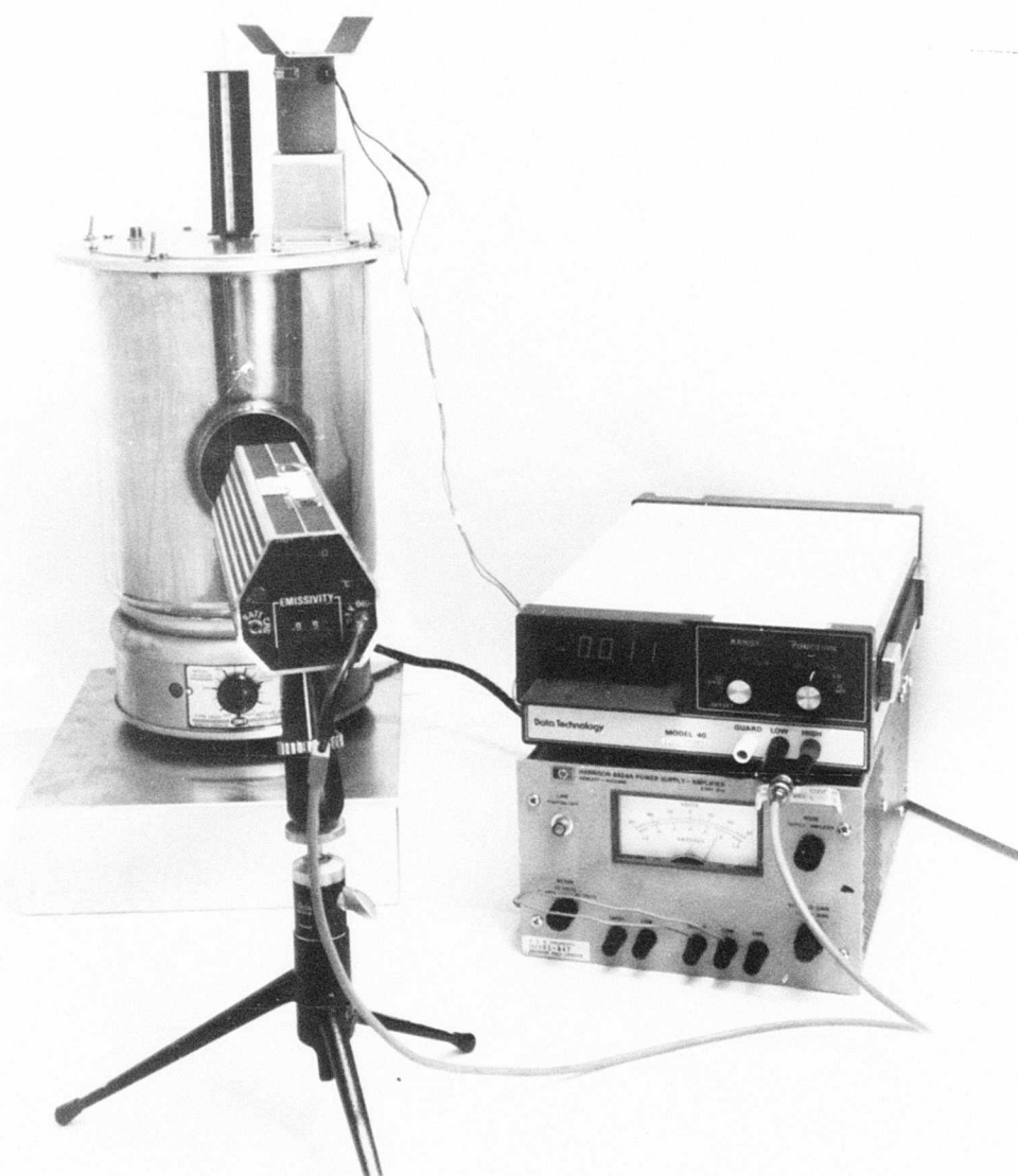
Figure 30 - Setup for Telatemp 44 Calibration
