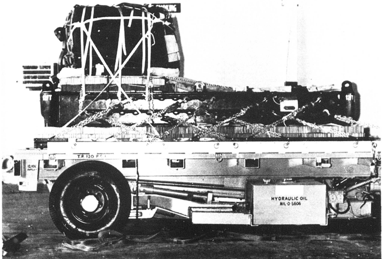
Figure 2. Two-Stage, Platform-Mounted, Multiple Recovery Parachute Airdrop System.
