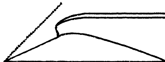
(c) SINGLE RAMP/CONE INLET.
