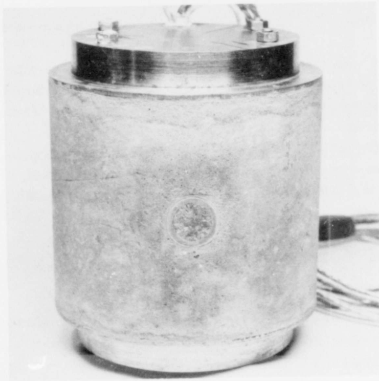
Figure 11. Concrete Sample Assembly
