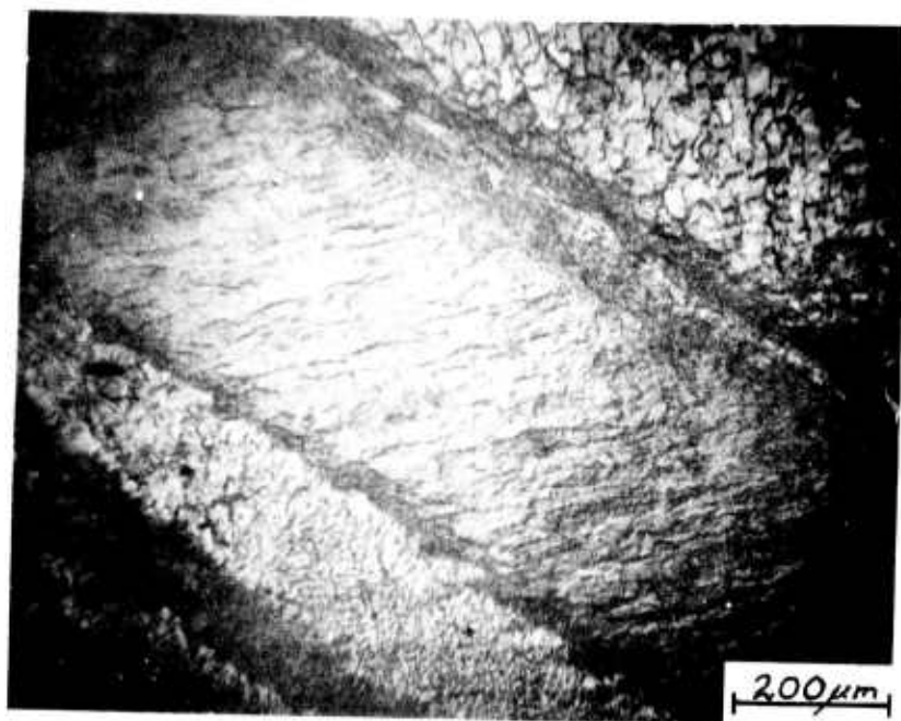
Figure E4. Inhomogeneous microstructure in \langle 111 \rangle sample forged at 0.56 T_m ( 640^\circ\text{C} ).
