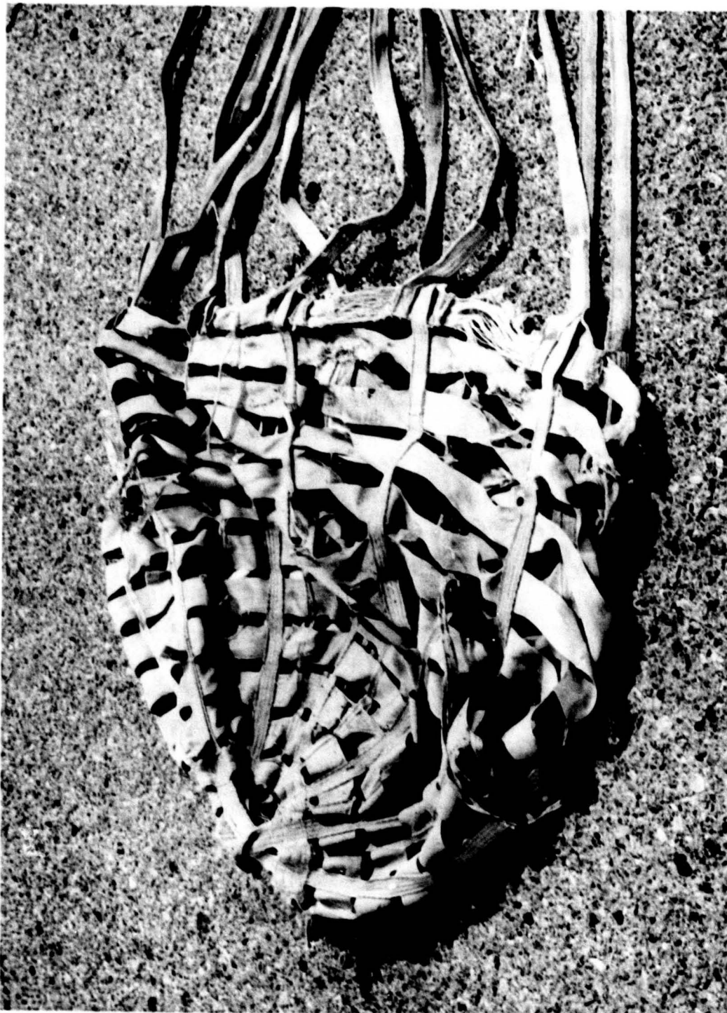
Figure 48. Post Test Photograph of the Test Parachute - Test 6P-G5.
