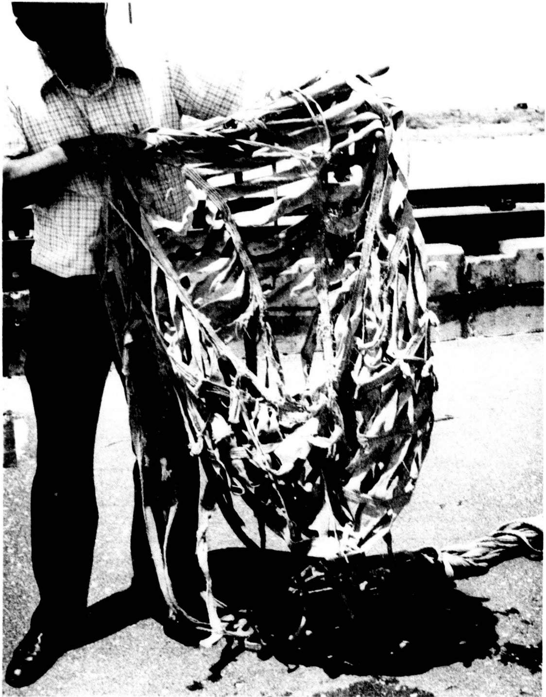
Figure 60. Post Test Photograph of the Test Parachute - Test 6P-H6.
