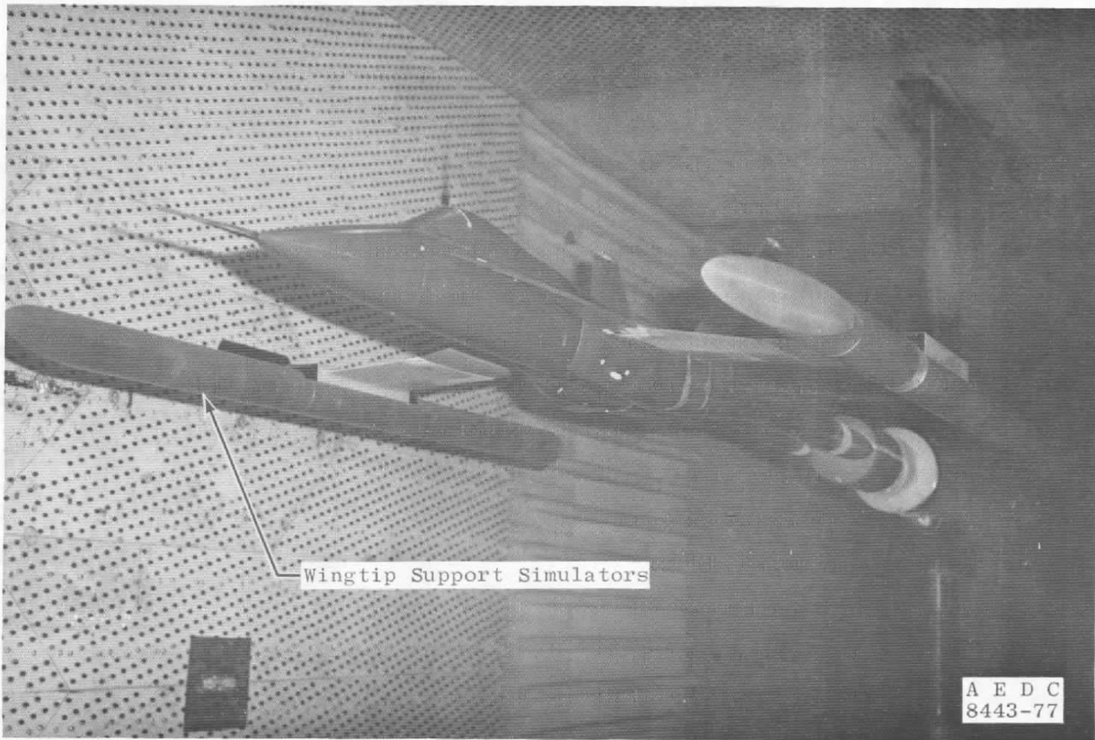
a. Phase I wingtip supports Figure 10. Wingtip support simulation.
