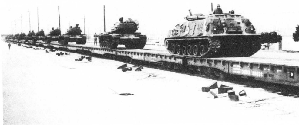
Figure 4-11. Circus-style rail loading of M88's and tanks.
