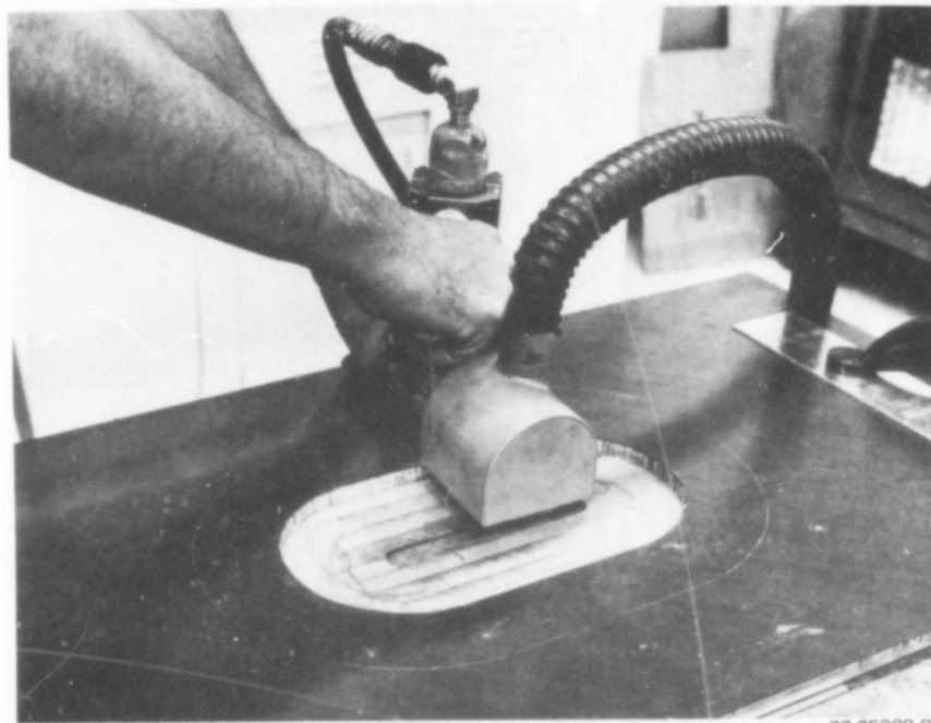
Figure 29. Scarfing the Inner Face of Panel Two
