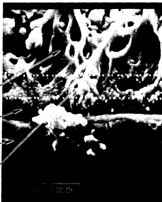
Figure E-18. SA-6029 Electroprimer on 10 Volt Phosphoric Acid Anodize Oxide Layers of Fractured -65F Tensile Shear Specimen B-2 in Apparent Adhesive Failure Area, 20,000X
