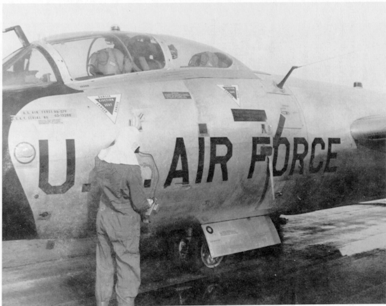
Figure 2.9 Radsafe monitor measuring exposure rate on a B-57 aircraft.
