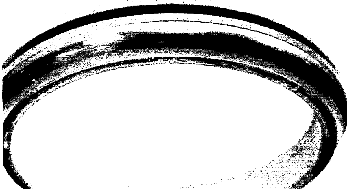
Figure 75. Loaded Inner Ring (TDC Coated) of 133-mm Bore Bearing After Component Test.
