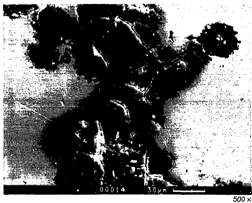
Figure 55. Corrosion Pitting on Ta + Implanted M50 Ball (Bearing No. 9 After 347 Hours). Note typical "mudcracking" in lower photo.
