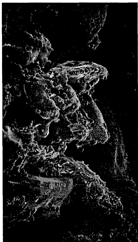
Figure 5B. SEM of PLGA after processing through a microfluidizer for 30 minutes. Magnification = \times 2000 ; [PLGA] = 0.1 g/L; solvent = isopropyl alcohol; pressure = 5000 Psi; method of cooling = ice bath
