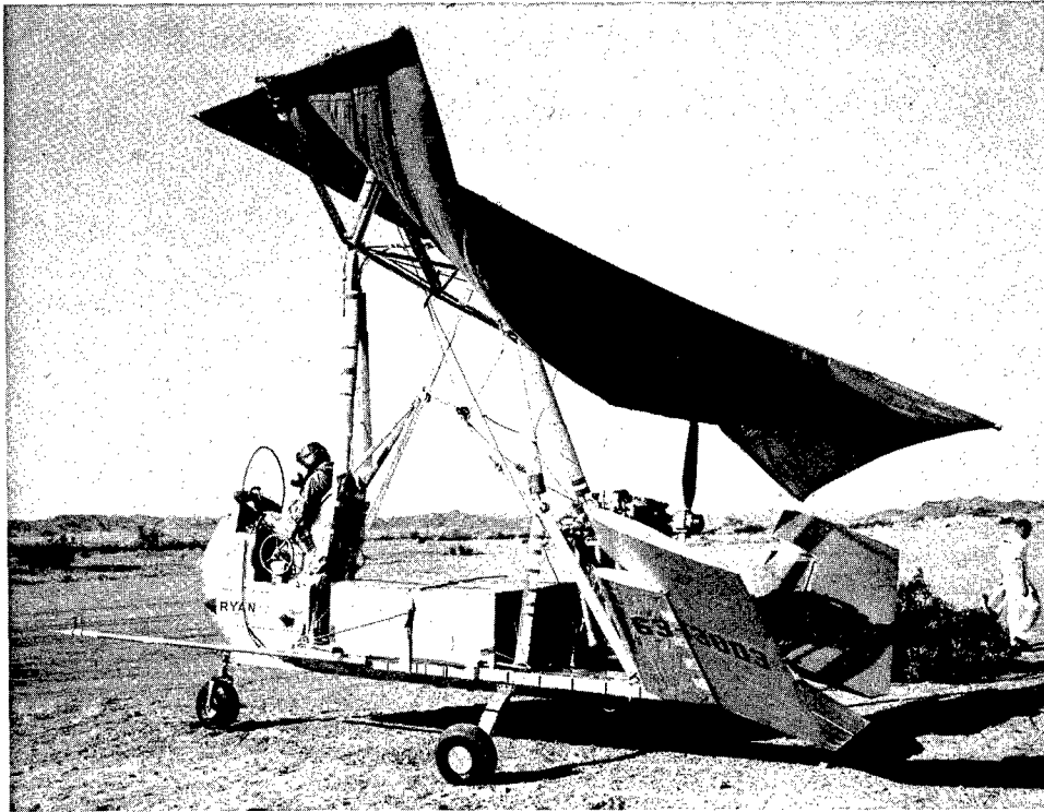
Figure 26. Medium Height Propeller Blockage Configuration
