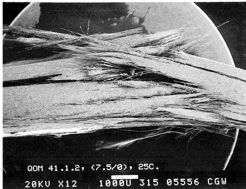
(A) VERY SPLINTERY FRACTURE AT 25°C
