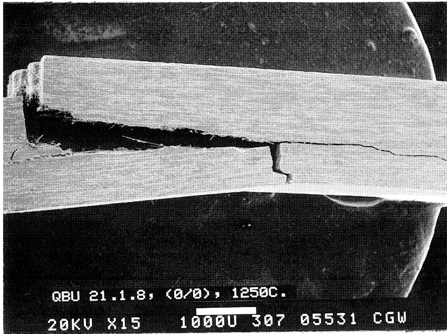
(C) 1250°C: NO DETECTABLE PERMANENT DEFORMATION
