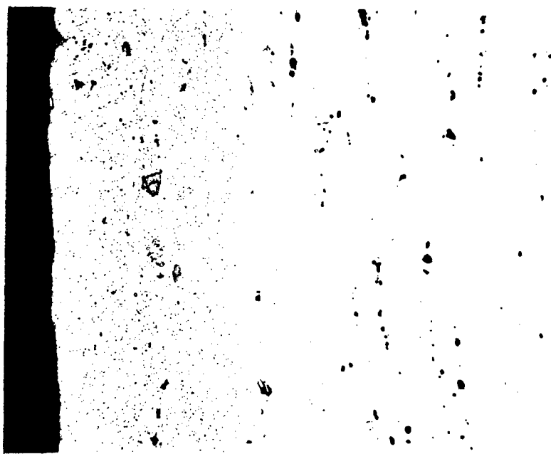
300X 0.5% HF 38080 Figure 3. Microstructure of Clad Spar Web (BMI 842-3) - Alcoa X76S type alloy (with high Cu) clad with 0.7% Si-0.5% Mn-1.0% Mg-Al base type alloy.
