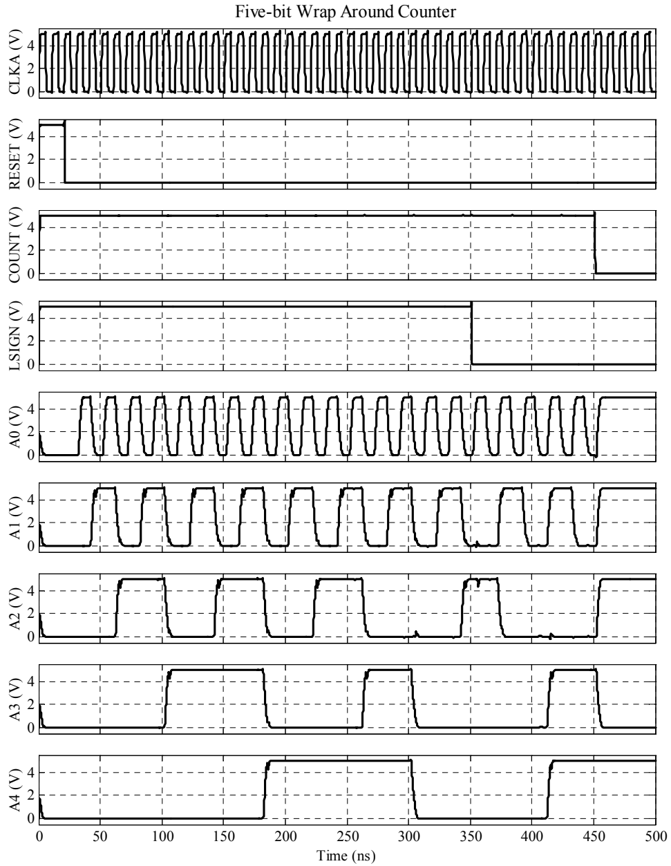
Figure 2.42 Five-bit wrap around counter simulation.
