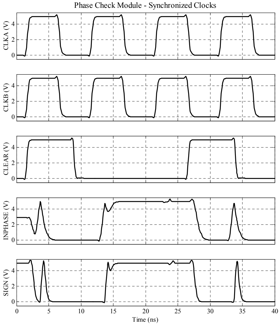
Figure 2.37 Phase-check circuit simulation – synchronized clocks.
