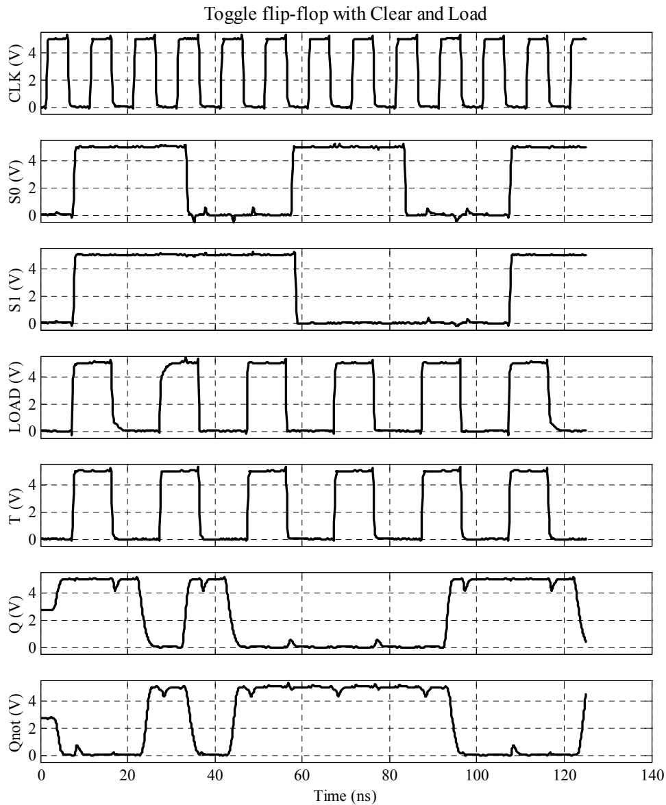
Figure B.11 Simulation results for the toggle flip-flop circuit.
