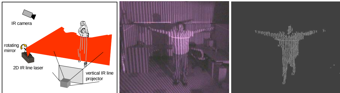
Figure 6: Dynamic scene capturing: (a) setup, (b) IR camera view with projected vertical stripes and the horizontal laser line, (c) reconstructed depth.
