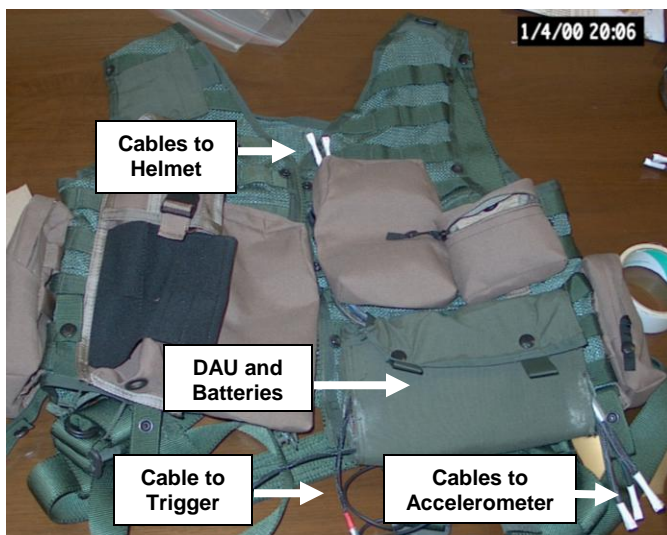
Figure 3. AIRSAVE vest with vibration equipment located in outside pocket
