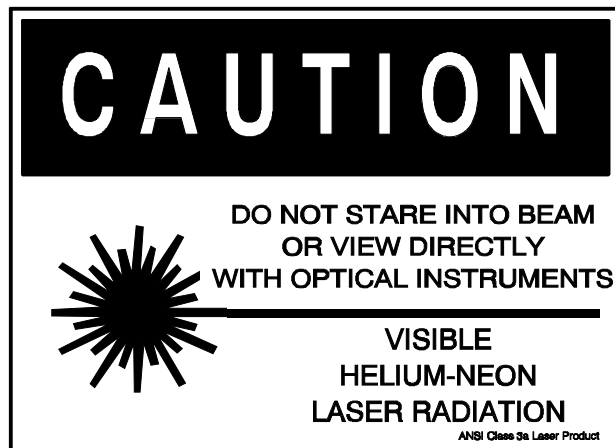
FIGURE A-1b. EXAMPLE OF A CAUTION LABEL FOR CLASS 3a VISIBLE AND NEAR-INFRARED LASERS
