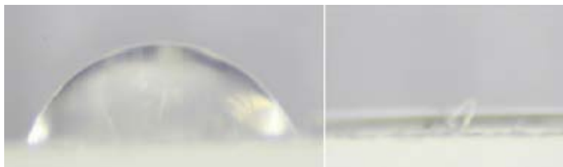
Figure 13. Water (left) and Dodecane (right) Droplets on an Untreated Nylon Film
