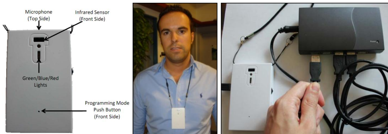
Figure 1: A diagram of a Sociometric Badge (left), a person wearing a Sociometric Badge (center), downloading data from the Sociometric Badges (right). Pictures are supplied by the SSI Sociometric Badge User Manual (Sociometric Solutions, Incorporated, 2011).
