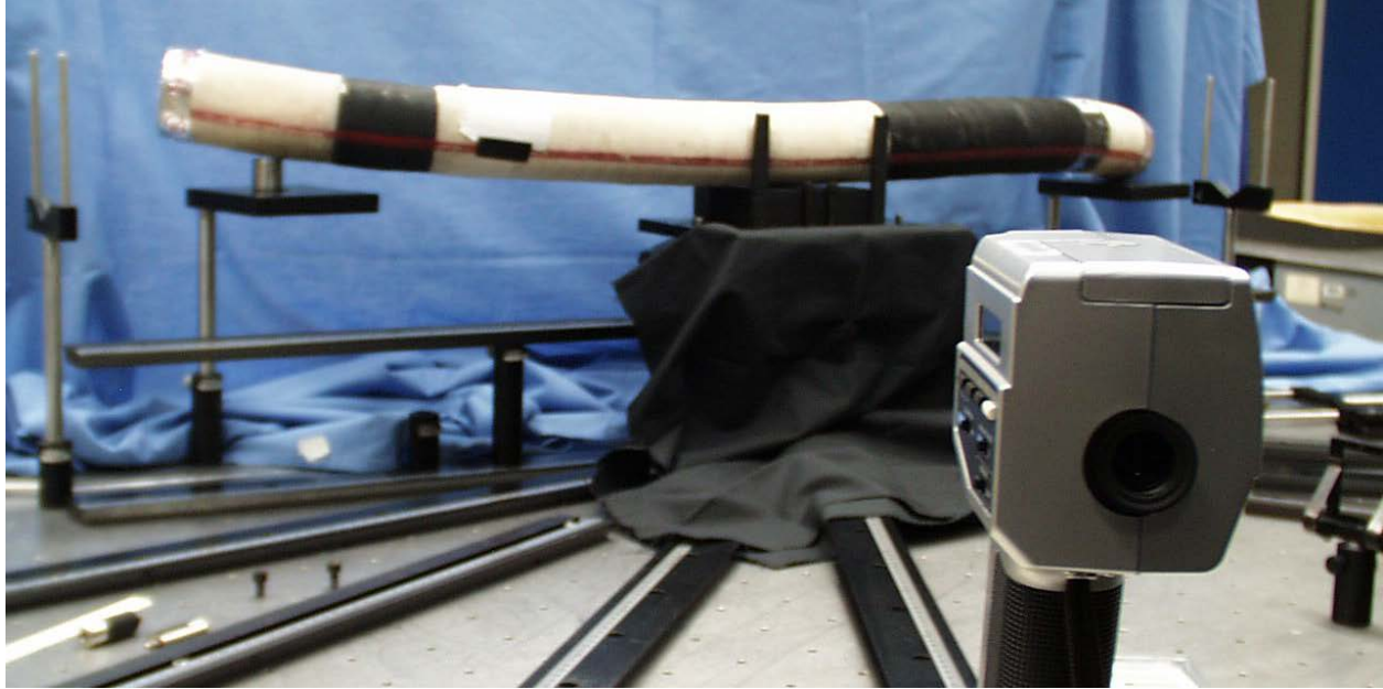
Figure 18. View From Behind the Photometer for White Portion of Hose Measurement at 60 Deg Angle
