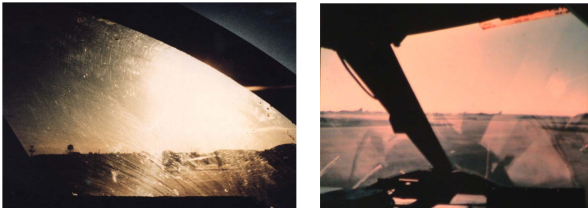
Figure 6. Loss of Contrast Due To Windscreen Haze (Left) and Reflections in the Windscreen (Right)
