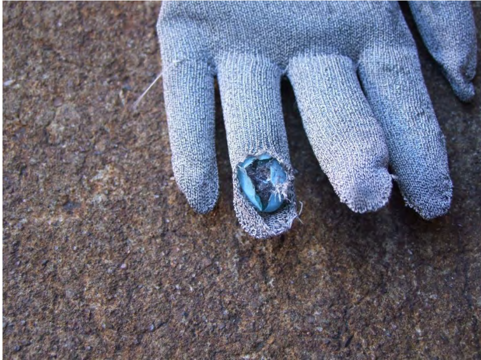
Figure A-9 Shows a Best T-Flex 8115 glove after detonation
