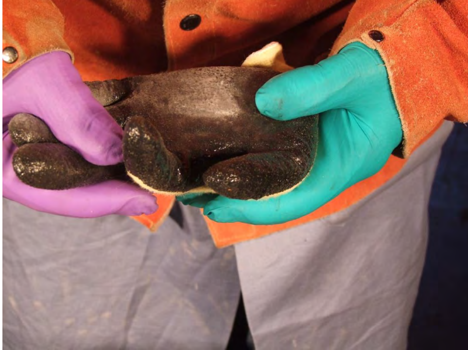
Figure A-5 Memphis UltraTech® 9693 glove after detonation, showing scorching
