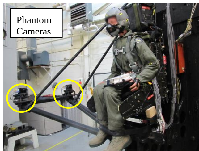
Figure 9. Phantom Miro-3 Cameras Mounted On-Board VDT Carriage
