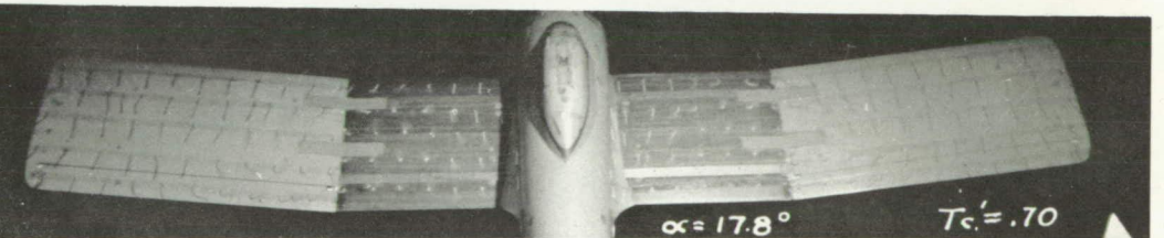
Figure 64.- Tuft study of \frac{1}{8} -scale model of Curtiss XBTC-2 airplane with rectangular wing; \delta_{f_1} = 0 , \delta_{f_0} = 0 ; slats closed; cowl flaps closed; L.G. up; take-off power.
