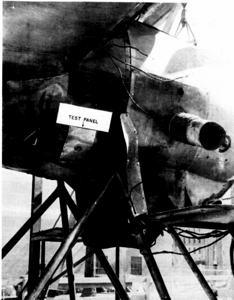
Figure 2. - Airplane subassembly used in the fire tests showing the location of a test panel in the nacelle skin. X1/12.
