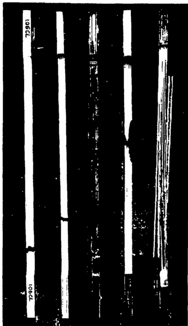
Figure 46.- Static tension creep specimens showing type of fracture; left to right, materials CL, G, R, P and G.
