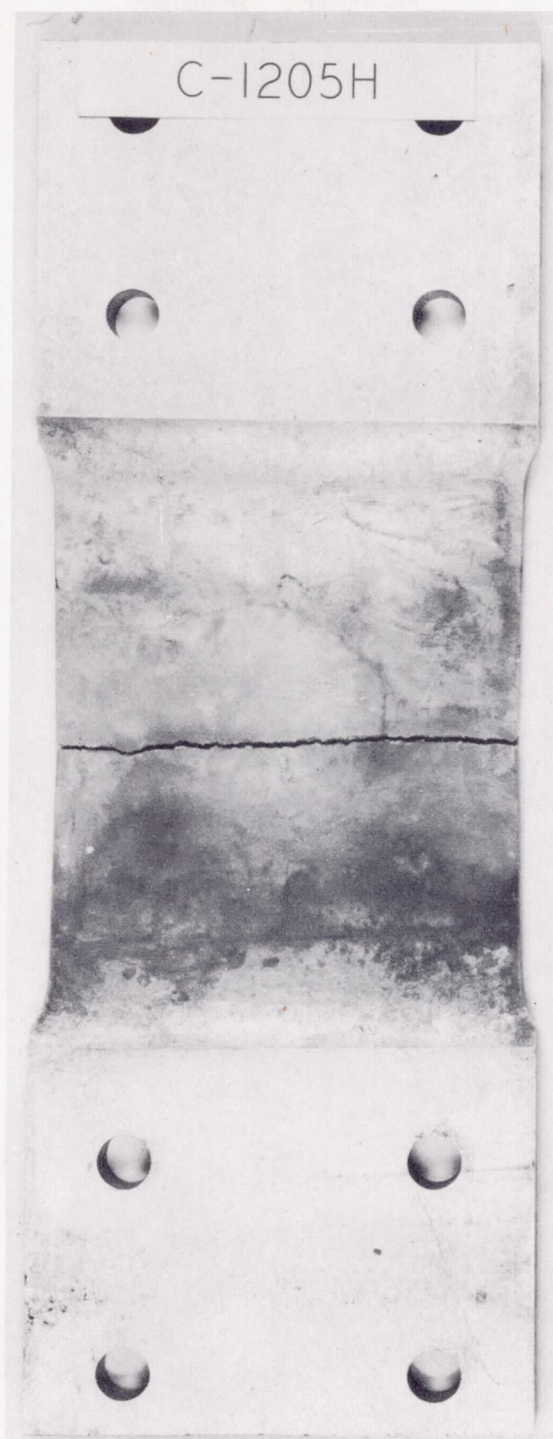
Figure 13.- Tensile failure of specimen not previously subjected to fatigue stressing.
