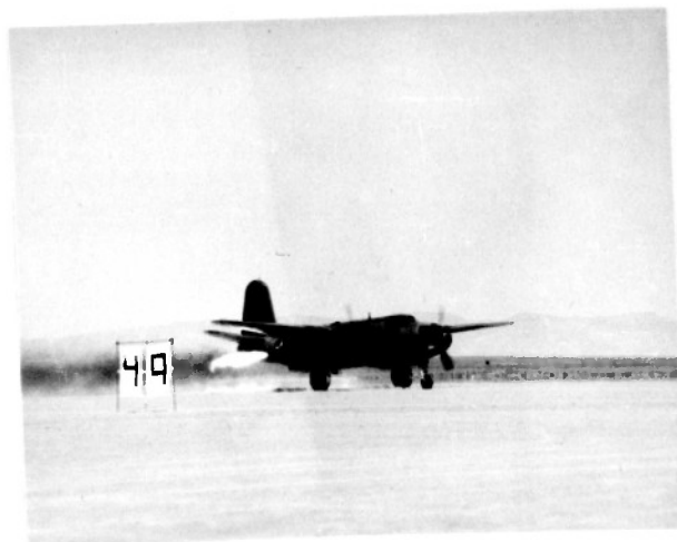
Fig. 28 -- Assisted take-off during ground run.
