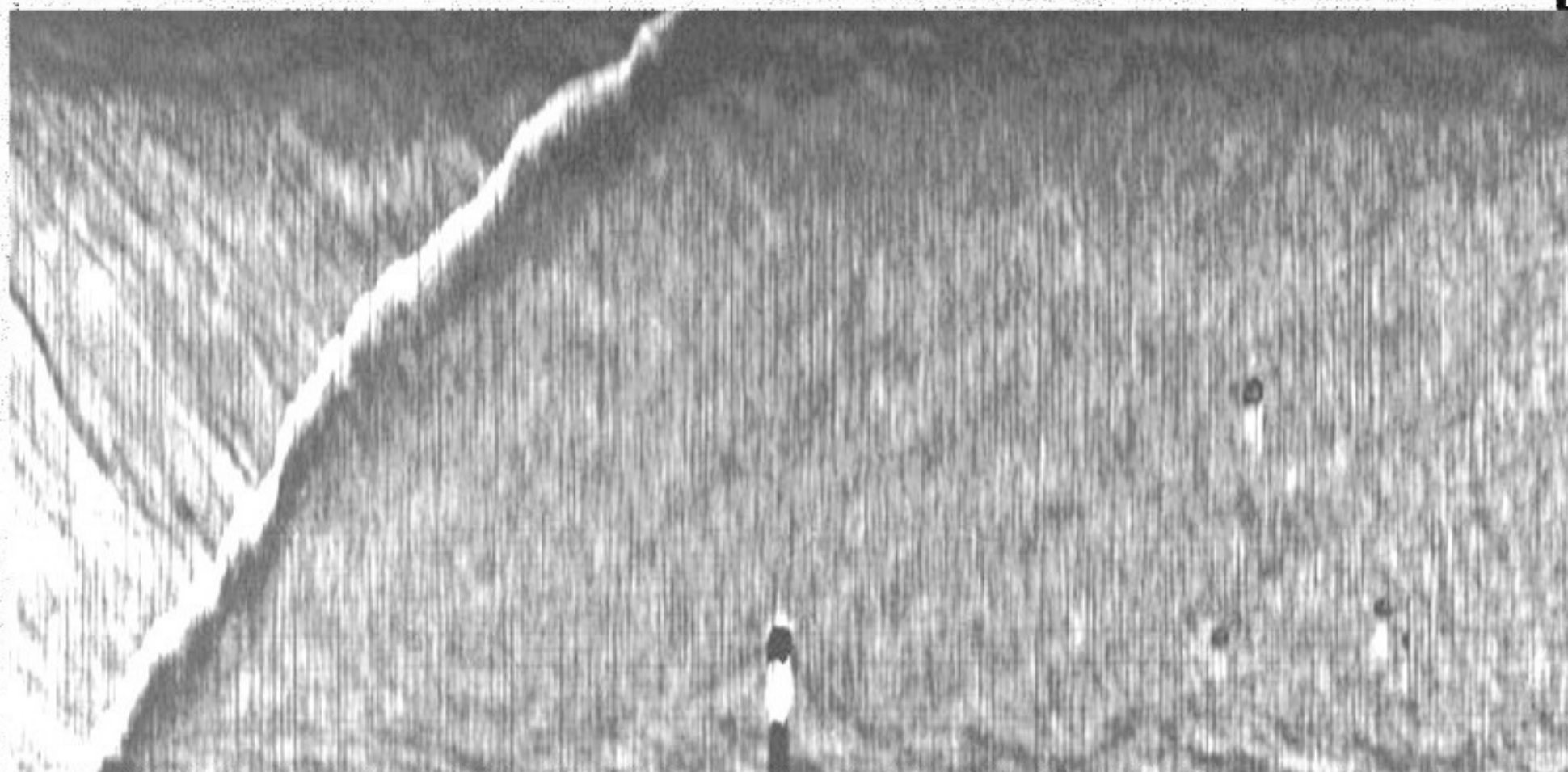
FIGURE 13 INFRARED PICTURE OF SCARS PRODUCED BY DROPPING THREE SIMULATED MINES NEAR AN OBSERVATION STAGE IN THE GULF OF MEXICO. THE WHITE LINE DEFINES THE EDGE OF A FAN-SHAPED SHEET OF WATER FLOWING OVER THE GULF FROM ST. ANDREW BAY. DATE: 5 MARCH 1964; TIME: 2204 S; COORDINATES: 30^{\circ}07'N , 85^{\circ}47'W ; AIRCRAFT ALTITUDE: 1600 FEET; LENGTH OF AREA SHOWN: 1.5 NAUTICAL MILES.
