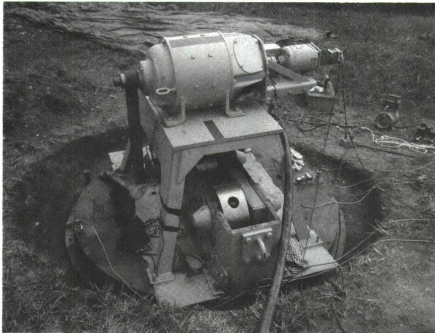
Fig. 2 - Vibration Generator and ground piston. The photograph was taken looking northeast and down, and shows the vibration generator, its drive motor mounted over it, and the ground piston installed in a shallow excavation needed to level the site. Five of the seven accelerometers mounted on the ground piston are visible in the photograph. One of the rotating masses in the vibration generator is visible at the nearer end of the generator. Photograph by Albert C . Grosvenor.
