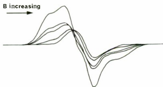
FIG. 4. Spectra from DGEBA cured with 70, 60, 50, 40, 30 p.b.w. DDM in solution, respectively.
