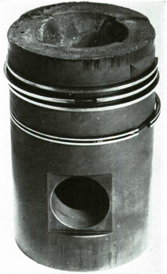
FIG. 5. Silicon nitride piston after trials.
