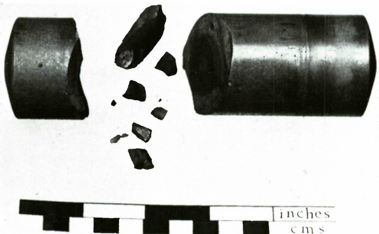
FIG. 6. Fractured silicon nitride gudgeon pin.
