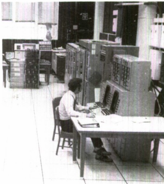
FIG. 2. The system certification and integration facility is a central computer complex for evaluating combat systems and components for new-construction submarines. The SCIF provides realistic at-sea simulations, such as sonar and periscope inputs.
