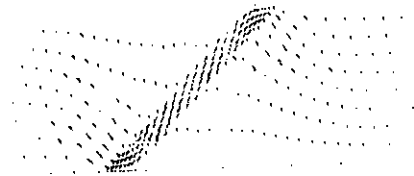
Fig. 2 Noninteractive example of grid adapting to prescribed pressure distribution with two degree of adaptive freedom.
