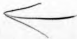
Fig.14: Wall streamlines near the beginning of a smoothly starting negative bifurcation line; numerical integration of equation (5) with a=0.5 , b=0.5 .
