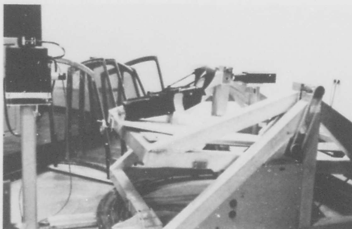
Figure 9. AFAMRL angular deviation measurement device and F-16 windscreen movement table with LANTIRN HUD
