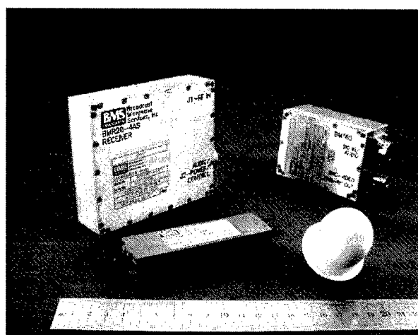
Fig. 6: Data link components and on board tracking Antenna
