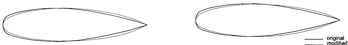
Fig. 22 - Shape of the modified airfoils for the untwisted (left) and twisted (right) wing, with l.e. radius constraint
