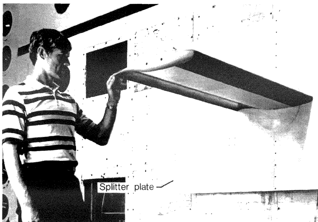
Figure 1. Rectangular supercritical wing installed in wind tunnel.
