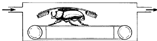
Figure 3. Measuring oxygen consumption of rhinoceros beetles carrying loads
