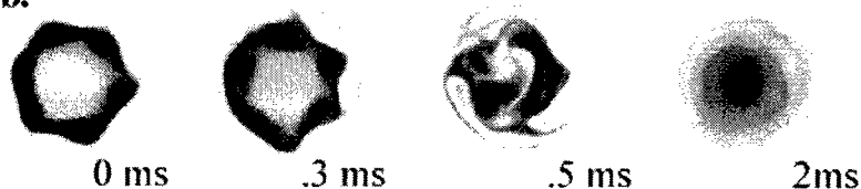
FIGURE 5. The progression of the diocotron instability a) in the presence of electron injection and b) without injection. Times shown are the time after the onset of the instability.
