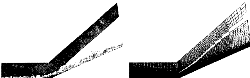
Figure 1. Typical instantaneous Mach number contours and shock-capturing stencils at the midspan location
