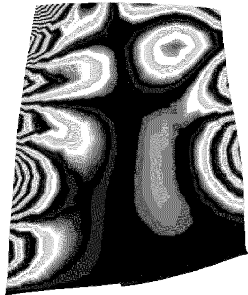
Figure 11: Calculated displacement field of mode no.20
