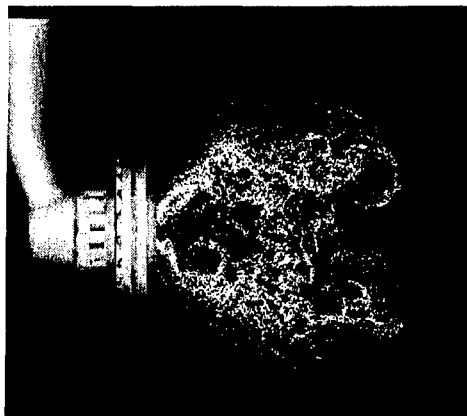
FIGURE 1. Snapshot spray from a gas-turbine fuel-injector.
