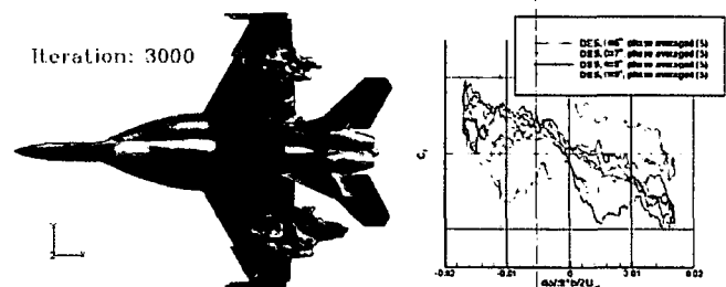
Figure 4. DES forced oscillations simulations. Left pane, instantaneous flow visualization at 6° pitch angle - contours of pressure on surface, and isosurface of zero streamwise velocity (grey). Right pane, rolling moment vs. roll rate phase averaged over 5 cycles.
