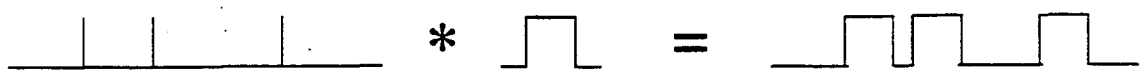
FIGURE 4. Transformation of a spike train-style waveform to a waveform that can be used for correlation by means of convolution with a simple response function.
